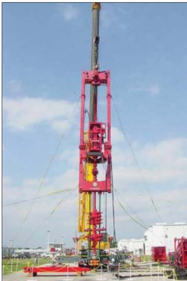
In a 2003 systems integration test in New Iberia, La., Halliburton checked a 4 1 / 16 -in. diameter, 15,000 psi BOP and a 135,000-lb coiled tubing injector head lift frame (Fig. 2; photo from Chevron).
