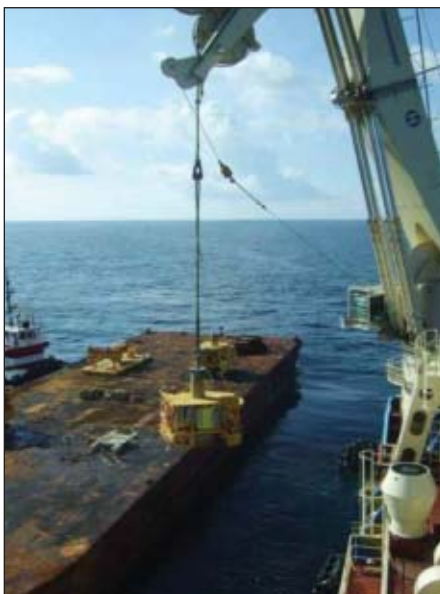
A Hydramarine crane on the MV Maersk Achiever lifts one of FMC's subsea trees from a transport barge for Chevron's Blind Faith project in the Gulf of Mexico (Fig. 1; photo from Chevron Corp.).
